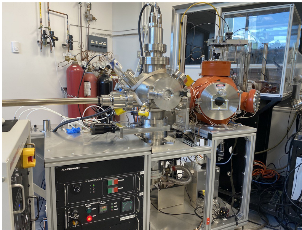
Figure 3.10: Pulsed laser deposition chamber (in orange) with load lock RF sputtering equipment (chamber to the right) used for this project.
